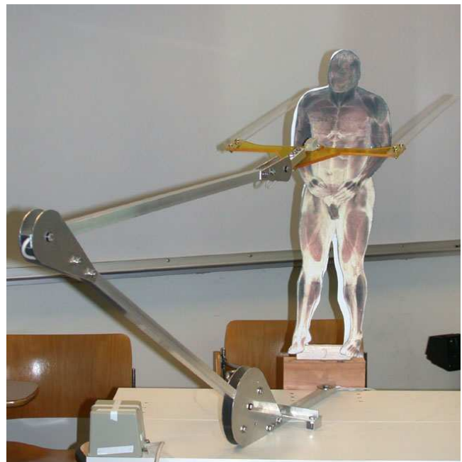
Figure 2: Design A consists of an adjustable arm, a fork representing the slice plane, and a 2D body.
